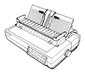
3. Lower the paper guide onto the back of the printer.
